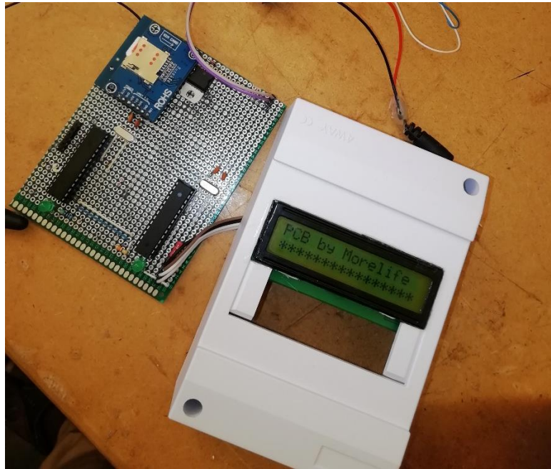
Figure Water meter PCB testing and In-Circuit Debugging
